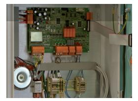
Developed with the latest technology in electronics components, it is fully integrated and easily accessible for maintenance and wiring. The weight measurement is done through top performance A/D converter used in the weighing systems. Input and output are protected from any wiring error and from electromagnetic noises, making these instruments really industrial.
