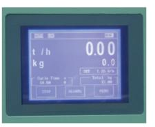
Use of touch-screen display make the operator interface extremely logical and user-friendly. Few and simple pressures on virtual buttons permit setting of main working parameters and detecting possible alarms. The head page reports evidently the decisive flow rate, net hopper weight and basic using indications.
