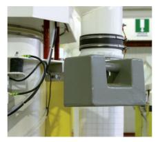
Calibration and periodical check can be easily and quickly executed by placing standard weights to the arms hinged on weighing hopper. Commands given through the operator panel allow to perfectly readjust the machine obtaining the required accuracy for effective control of plant yield.
