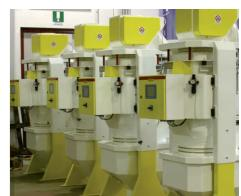
In the age of communication systems we cannot ignore this nowadays fundamental aspect. Three communication field busses are available: Profibus DP / Modbus / TTY (current loop). PES scales are perfectly integrated in new automation systems and in existing ones, allowing the replacement of existing flow control systems.
