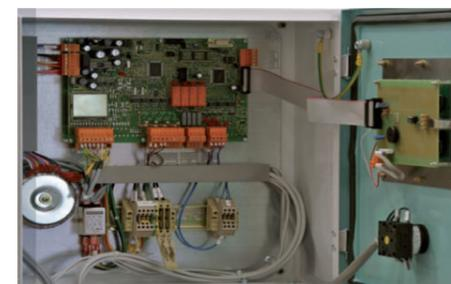
Developed with the latest technology in electronics components, it is fully integrated and easily accessible for maintenance and wiring. The weight measurement is done through top performance A/D converter used in the weighing systems. Input and output are protected from any wiring error and from electromagnetic noises, making these instruments really industrial.
