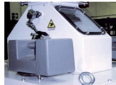
Calibration and periodical check can be easily and quickly executed by placing standard weights on the disks assembled to the weighing hoppers. Commands given through the operator panel allow to perfectly readjust the machine obtaining the required accuracy for effective control of plant yield.
